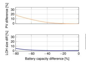
PV and H<sub>2</sub> evolution, depending on the battery capacity reduction. The reduction is computed on the basis of the reference configuration.
