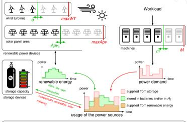
outputs: configurations (m, q, Apvq, storage capacity) + associated metrics, QoS, etc.
