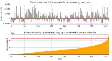
Electrical sizing on Minneapolis (USA) - 2021, for the configuration (WT, PV) = (4, 3277)
